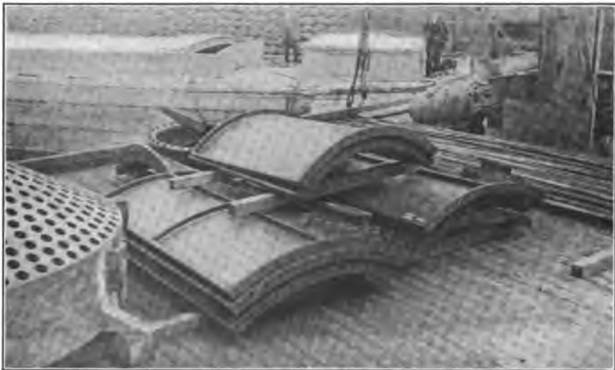
FIG. 136.—Portions of belt of a 10 ft. 6 in. diam. vacuum pan. The larger pieces are 5 ft. 6 in. \times 9 ft. 0 in. \times 1 ft. 0 in. and weigh 2,200 lb. each.
